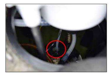
Note the correct positioning of the fuel level sensor float.
