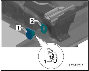
• Reinstall the seat rail stop bolts <2> (if removed). Tighten the bolts to 20 Nm.
