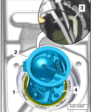
Reconnect the fuel pump connector to the fuel filter flange.
