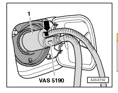
Reinstall the fuel filter flange locking ring by turning clockwise. Torque the locking flange to 110 Nm.
