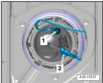
• Move the fuel pump flange into the installation position.
