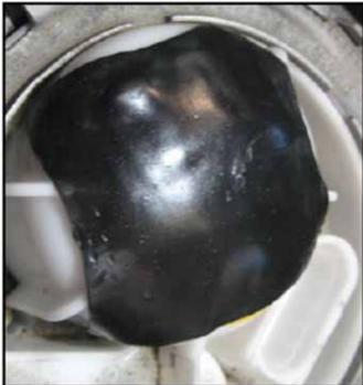
If there are NO cracks and/or yellow • discoloration present, apply the protective film as shown in the next step.
