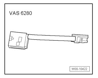
• Airbag Lockout Connector -VAS 6280-
