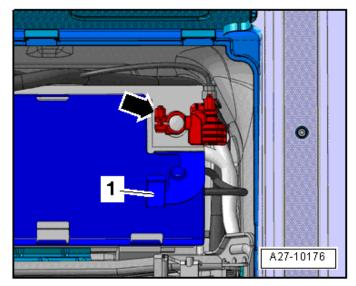
Unlock the retaining tabs <arrows> and open • the cover <1>.
