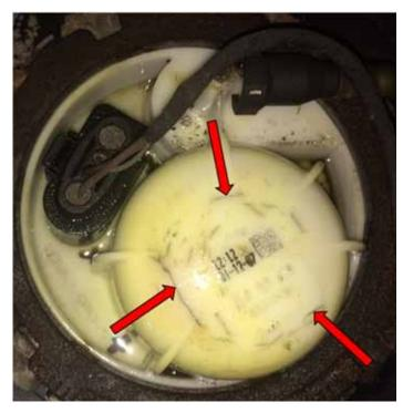
Remove the fuel pump flange cover <1> by removing the three screws <arrows>.
