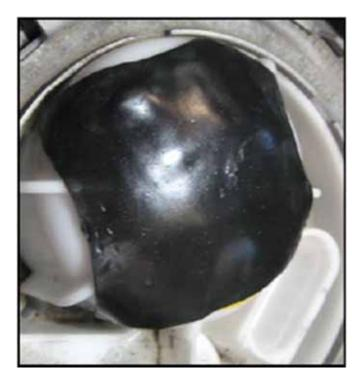
Apply protective film as shown. Start • application from the center and work the protective film towards the outside edges of the fuel pump flange taking care to eliminate air gaps or bubbles under the film.
