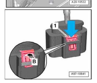
Be sure to properly engage the red locking tab <1> by pressing down <arrow> after properly securing the connector.
