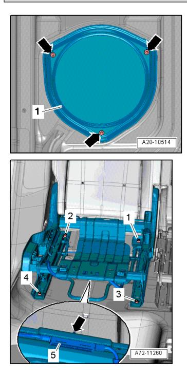
Reinstall the fuel pump cover <1> by installing and tightening the three screws <arrows>.
