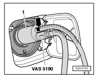
Dispense recovered fuel contained in the -VAS 5190- Fuel Extracting Device back into the vehicle fuel tank.
