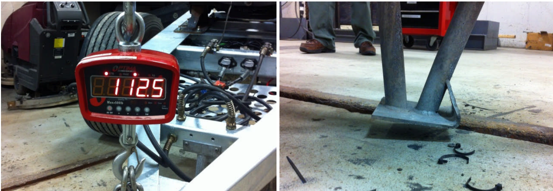
18. Hang a scale from the hoist and connect to the eye with a chain. Using the hoist, suspend the front of the dolly with the jack stand approx 1" off the floor.
