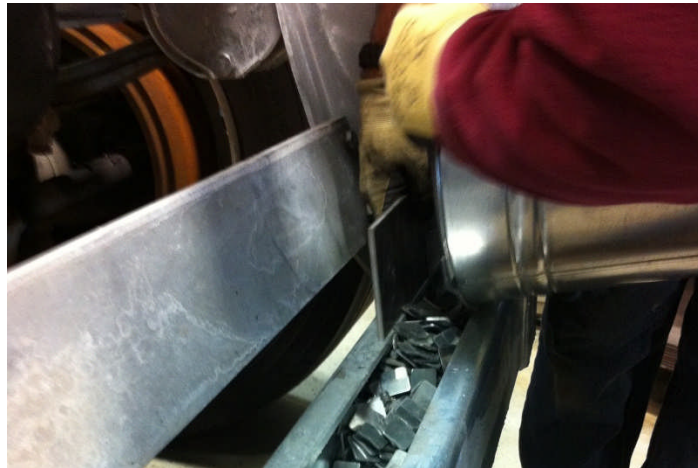
19. Completely fill the lower bumper channel with galvanize slugs for counter weight.
