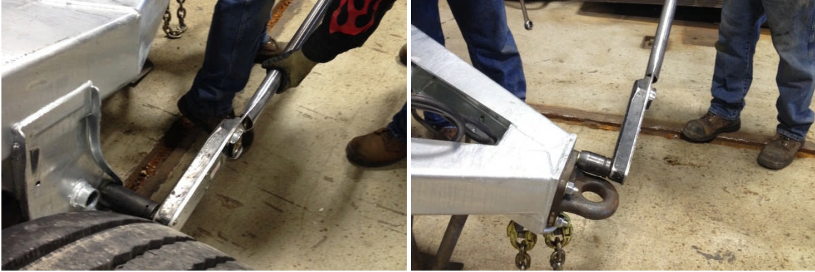
17. Torque the torque arm bolts to 550 ft. lbs. Torque the eye bolts to 275 ft. lbs.
