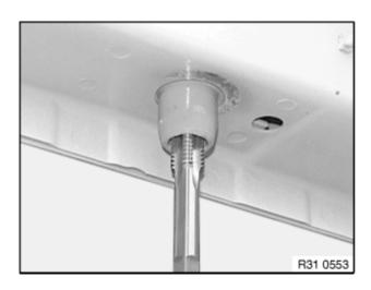
2. Create locating thread for Helicoil thread insert
