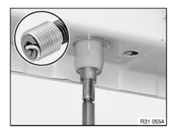
3. Use Helicoil thread insert M12x1.5x30 and screw into the locating thread until flush with the original thread
