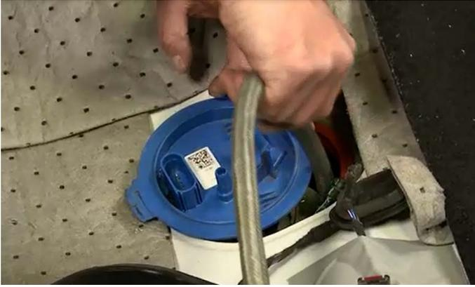
Use cold weather protective gear or equipment as necessary, drain all of the fuel out, or warm the vehicle indoors if the vehicle has been stored in an extreme climate condition before performing the next steps.
