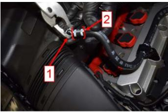
Install the new spring clamp <1> onto the outlet side of the new fuel line, centering it in between the white lines which show proper clamp location <2>.
