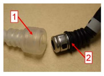
Install the translucent cover <1> onto the chassis side metal fuel delivery line in the orientation shown and push it down the metal fuel delivery line far enough as to not interfere with the fuel line push-lock connector <2> installation.
