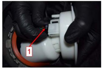
Plug in the fuel pump connector <1> until it seats properly and the locking tab has clicked in place.
