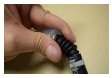
Squeeze, pinch, and pull on the translucent cover as shown to guide it into position past the sealing ring on the fuel line push lock connector.
