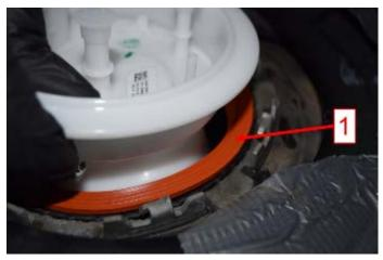
Properly seat the flange seal ring <1> into the fuel tank and verify that the seal is properly seated before applying pressure to the top of the locking flange to seat.
