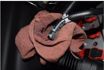
Put a rag or other absorbent material around the base of the fuel line outlet and pull and twist on the line to remove it from the fuel pump nipple. Catch as much residual fuel as possible using the rag or other absorbent material.
