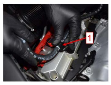
• Install the new fuel line, starting with the securing loop <1> on the upper right hand side of the right valve cover.
