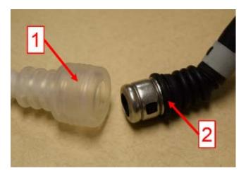
Unseat the translucent cover <1> from the fuel line push lock connector seating ring <2> and push it up the chassis side metal fuel delivery line far enough to not interfere with disconnection of the fuel line push lock connector.
