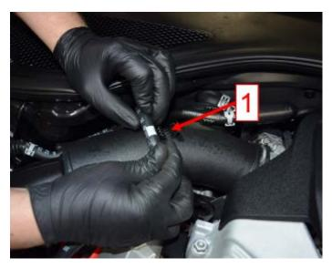
Secure the fuel line into the securing hook on the air inlet tube <1>.
