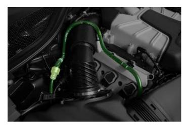
Locate the under hood fuel line on the right side (passenger side) of the engine compartment. The line inlet is located near the firewall behind the air box, and the outlet is located in front of the right side valve cover at the top of the high pressure fuel pump.
