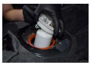
Pull the locking flange out of the opening in the fuel tank and tip the fuel delivery unit to assist in draining as much fuel from the fuel delivery unit as possible.
