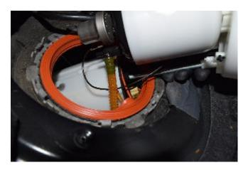
Tip the fuel delivery unit as shown in the photo to empty as much fuel as possible from the delivery module before attempting removal.
