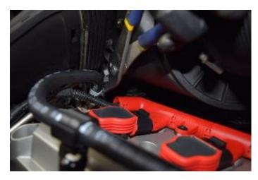
Using one hand, squeeze the pliers and open the clamp. Use your other hand on the fuel line to guide the line onto the fuel pump nipple. When the line is seated, release pressure on the pliers to secure the clamp.
