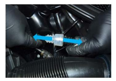
Pull gently apart on the metal chassis fuel delivery line and the newly installed rubber fuel line to verify a secure connection <arrows>.
