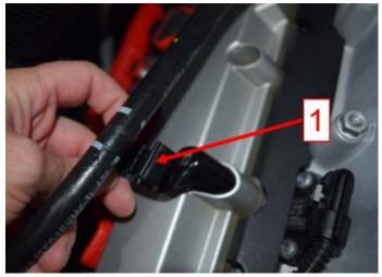
Unclip the securing loop <1> located on the upper right side of the right hand valve cover.
