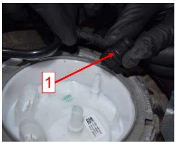
Install the closure cap <1> onto the small connector on the top of the new fuel delivery unit.
