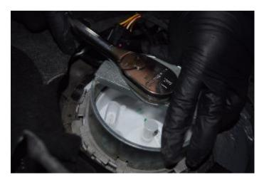
Install the locking ring using the -T10202-Locking Ring Flange Tool.
