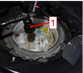
Remove the fuel line connector <1> from the locking flange by squeezing the release tab between the finger and thumb, pushing down on the connector, then lifting up.
