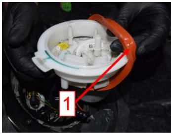
Dislodge the seal <1> from the tank opening and carefully remove it over the top of the locking flange.
