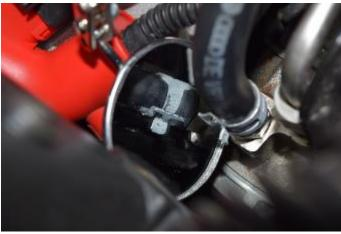
Use a dentist's mirror (or similar) to verify that the line has been completely seated, and that the clamp is securely fastened in between the white lines on the fuel hose indicating the correct position of the clamp.
