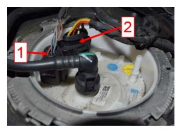
• Disconnect the connectors <1> and <2> on the locking flange of the fuel delivery unit.
