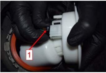
Disconnect the fuel delivery unit electrical connector <1>.
