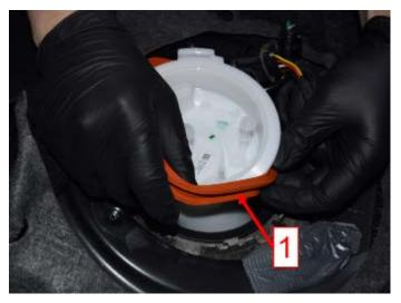
Install a new locking flange seal <1> by working the seal over the top of the fuel pump flange.
