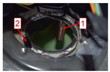
• Carefully remove the fuel delivery unit through the opening in the fuel tank.
