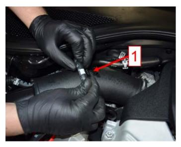
Unclip line from the securing hook <1> on the air inlet tube.
