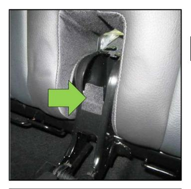
Apply a section of felt tape (approximately 35mm x 40mm) to the seat frame in the area shown <arrow>.
