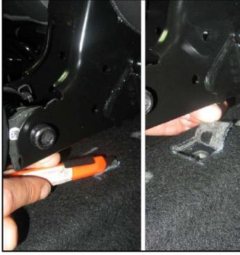
• Using a utility knife (or equivalent), cut the outlined area of the carpet (35mm x 35mm).
