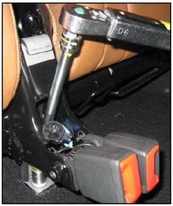
Install the support bracket into the seat frame.
