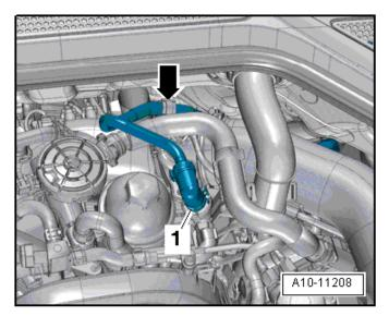
Reconnect the vacuum hose <1> and place back in bracket <arrow>.
