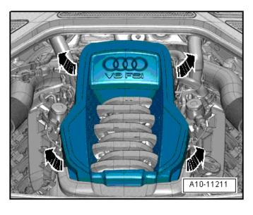
Reinstall the engine cover by first pushing the engine cover with both hands into the rubber grommets in the rear and then into the rubber grommets in the front.
