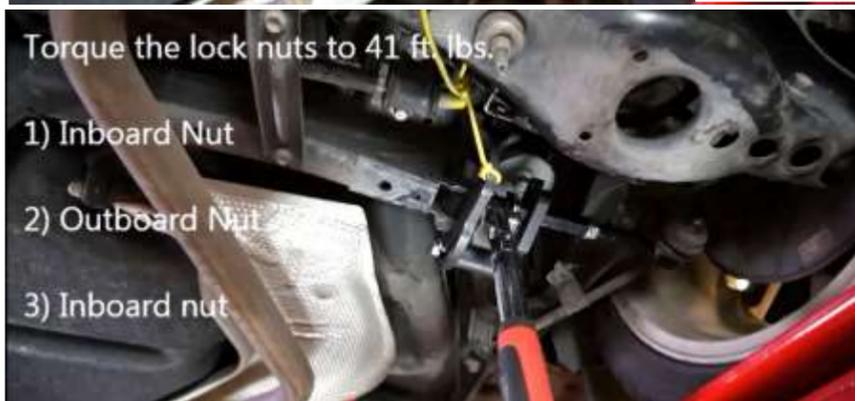
Torque the lock nuts to 41 ft. lbs.
