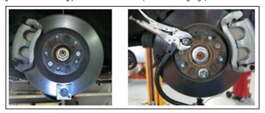
10. Place the sensing tip of the dial gauge on the bottom of front lower arm ball joint (A) as shown below:
