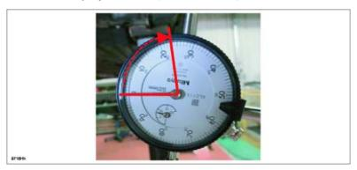
**NOTE:** If dial gauge scale does NOT return to 0 mm {0 in.} when release the pry bar, it is NOT being measured correctly. Re-start the inspection procedure step 9.
