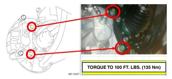
**STEP 3:** Using a 14mm socket, 3/8" swivel adapter and a 3" extension, verify the torque of the 8- (4 each side) 14mm hex head bolts securing the front hub unit to the axle housing. **Torque each bolt to 70 ft. lbs. (95 Nm).**
