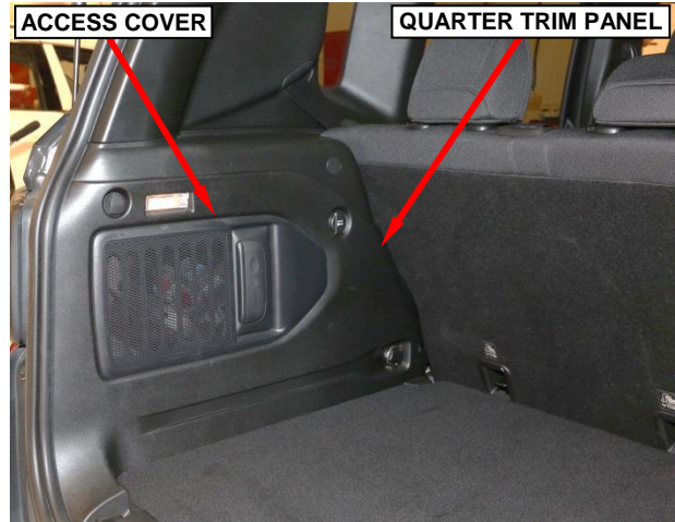
Figure 2 – Quarter Trim Access Cover
