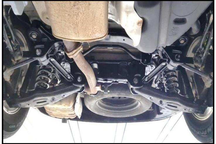
2. Check for complete welds in the locations (1) and (2) shown in the illustration on both sides of the cross-member. Check to see if the welds are broken, misaligned or missing.
