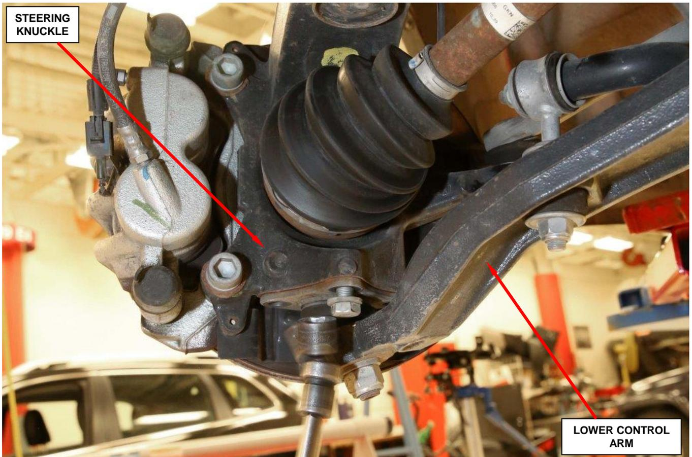
**Figure 24 – Three Ball Joint Retaining Bolts**
