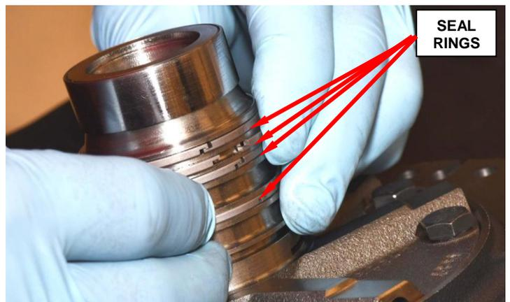
**Figure 37 – Oil Pump Seal Rings**
