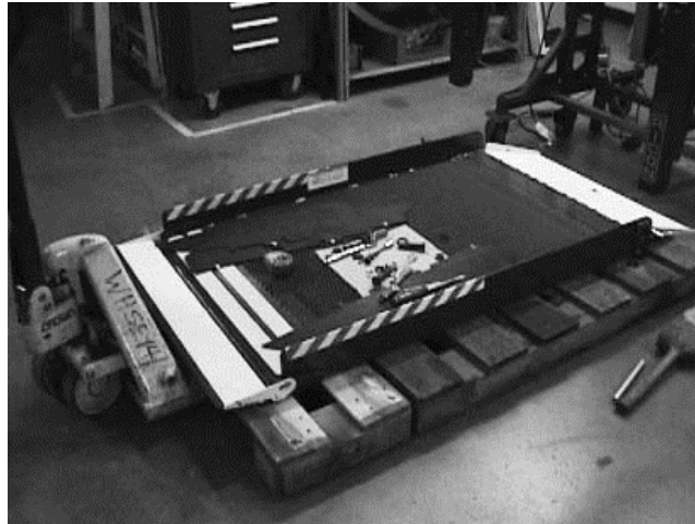
Figure 16. Discard Damaged Platform
