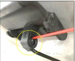
2. Verify proper operating of secondary hood latch. Wipe off any excess lubricant.
