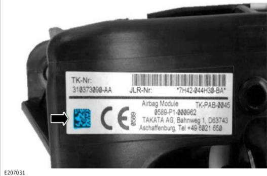
Locate the QR code on the NEW passenger airbag module label.
