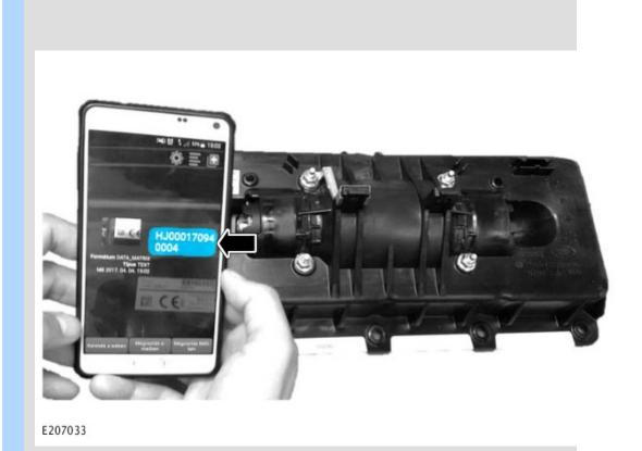
Use a smartphone with a QR code scanner to scan the QR code of the NEW front passenger airbag module.
