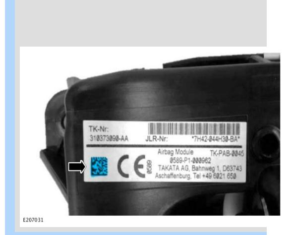
Locate the QR code on the NEW passenger airbag module label.
