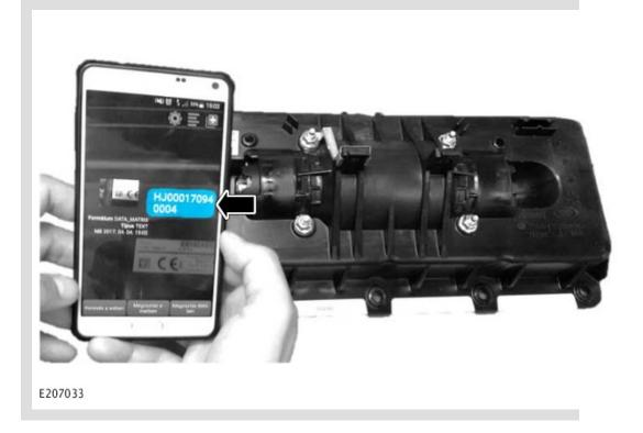
Use a smartphone with a QR code scanner to scan the QR code of the NEW front passenger airbag module.
