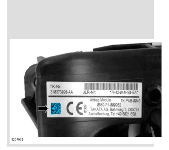
Locate the QR code on the NEW passenger airbag module label.
