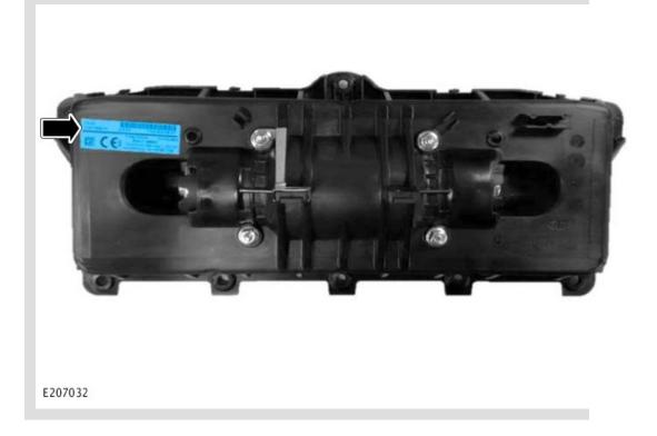
Locate the label on the NEW passenger airbag module.
