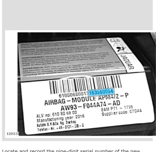
Locate and record the nine-digit serial number of the new airbag module on the claim verbatim.
