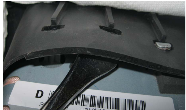
Retaining claws being CAREFULLY disengaged.
