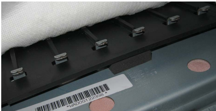
Module in position, retaining claws engaged.
