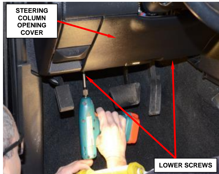
Figure 4 – Steering Column Opening Cover
