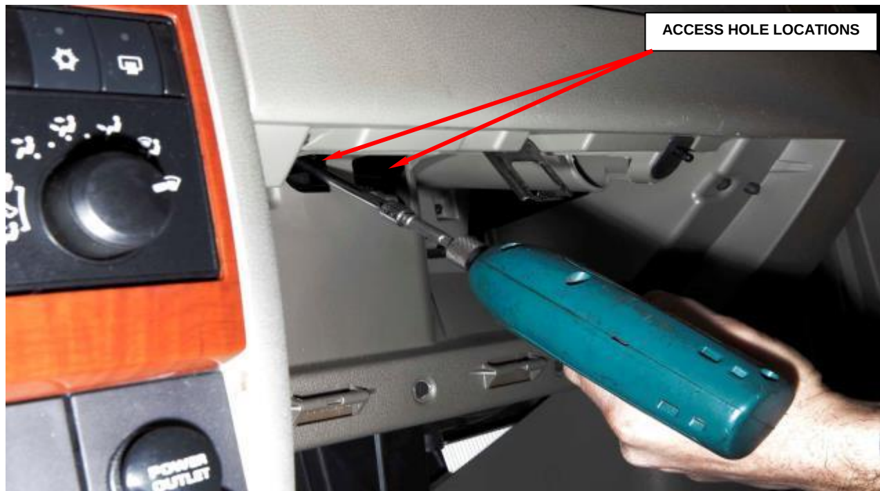
Figure 47 - Passenger Airbag Mounting Bolt Access Holes
