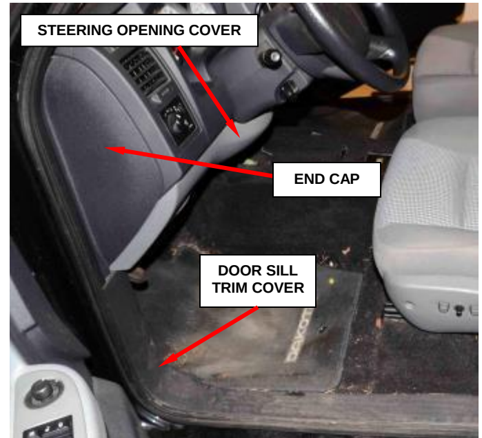
Figure 130 – Door Sill Trim (Driver Side Shown)
