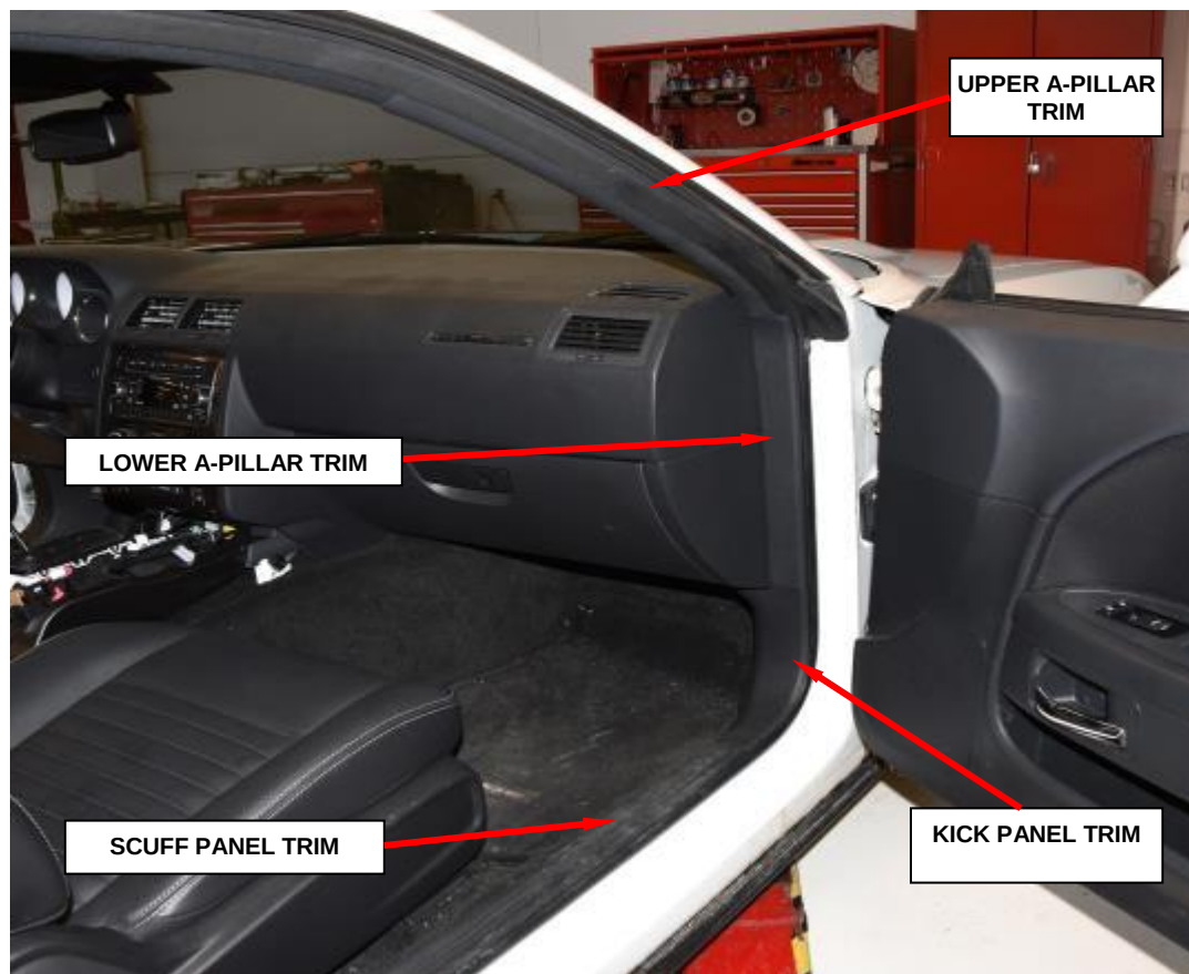
Figure 92 – Door Opening Trim (Right Side Shown, Left Side Similar)
