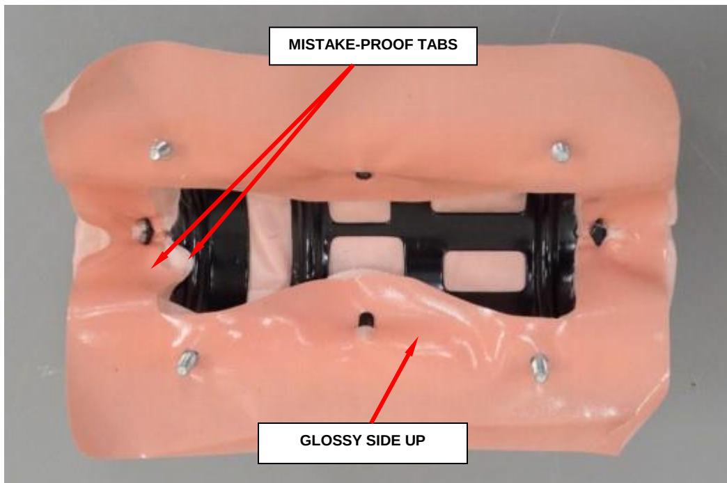
Figure 155 – Fabric Gasket to Cushion (Glossy Side Up)
