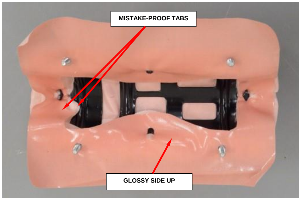
Figure 124 – Fabric Gasket to Cushion (Glossy Side Up)
