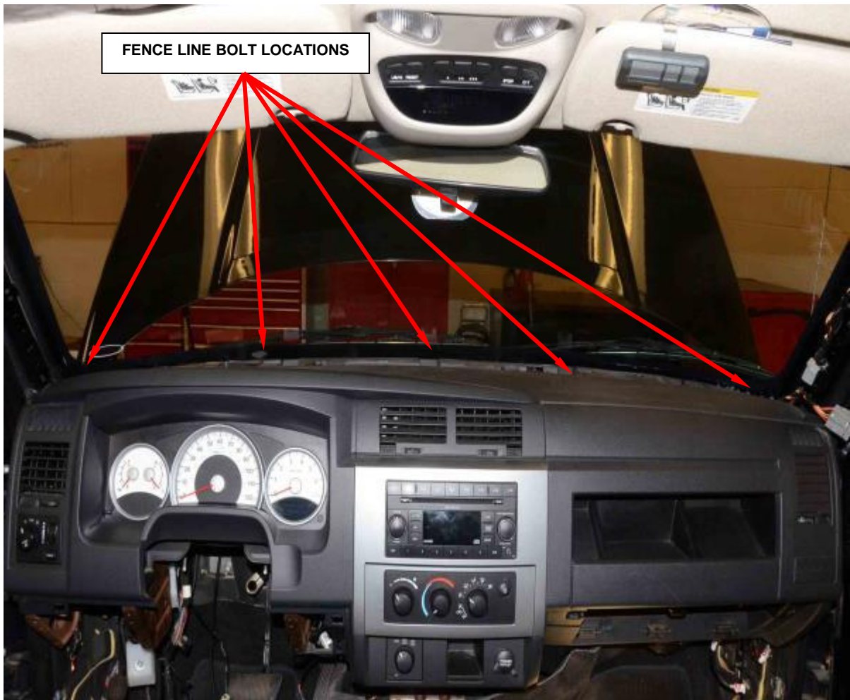
Figure 115 - Fence Line Bolts
