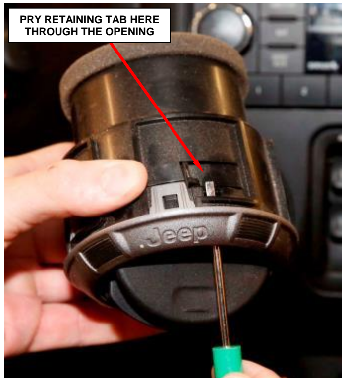
Figure 131 - HVAC Outlet Tab
