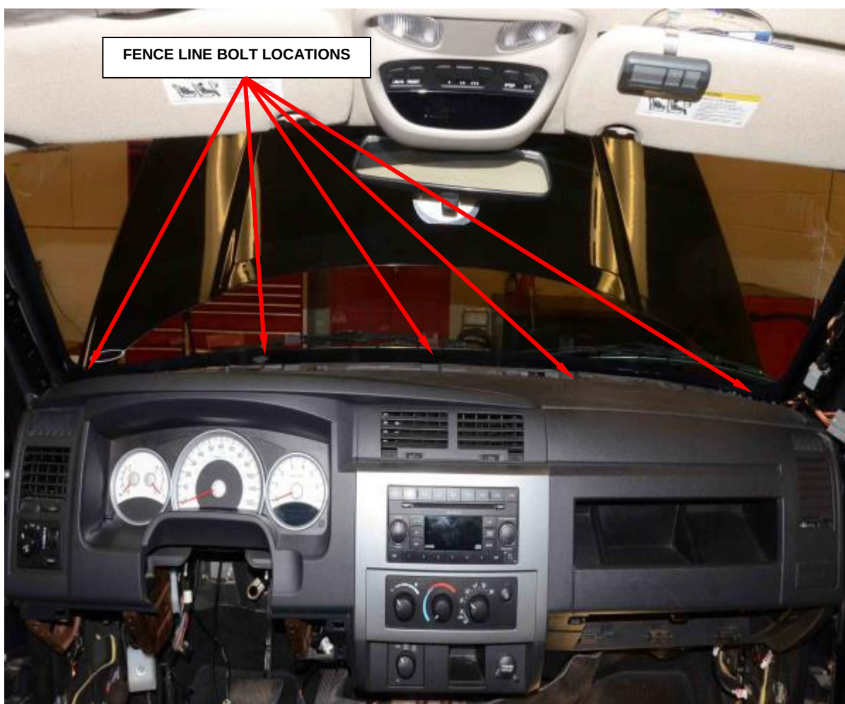
Figure 140 - Fence Line Bolts
