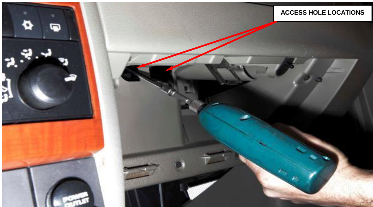
Figure 42 - Passenger Airbag Mounting Bolt Access Holes
