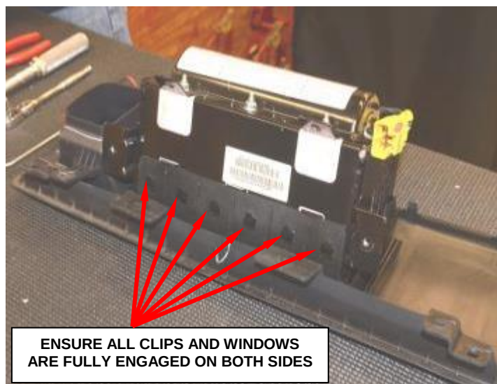
Figure 29 – Airbag Cover and Airbag Module
