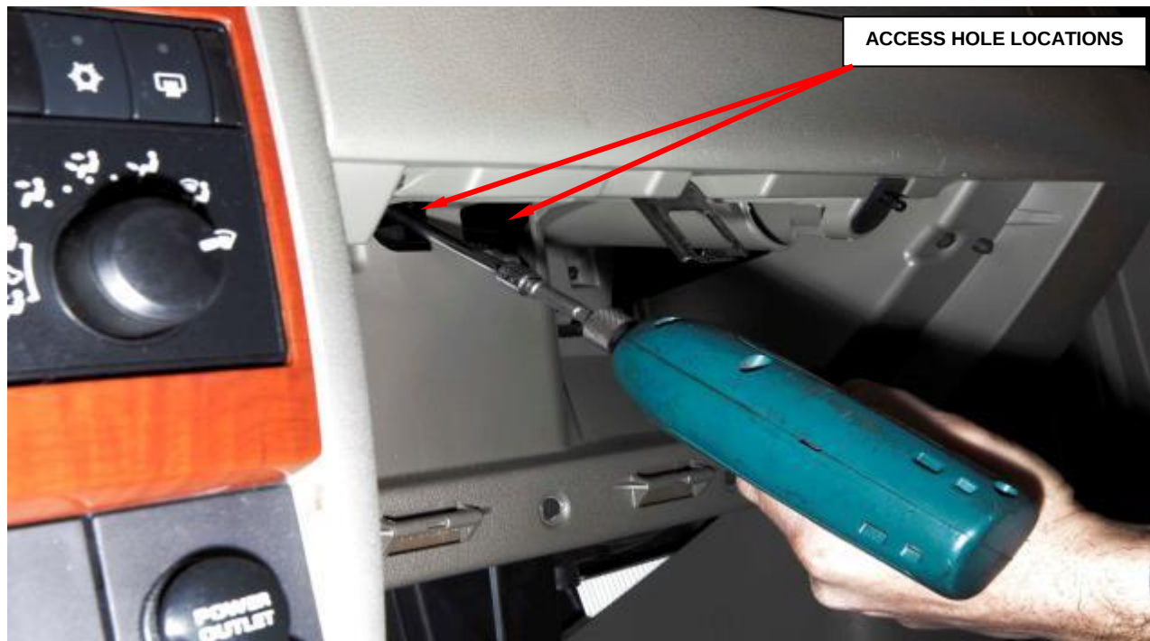
Figure 47 - Passenger Airbag Mounting Bolt Access Holes
