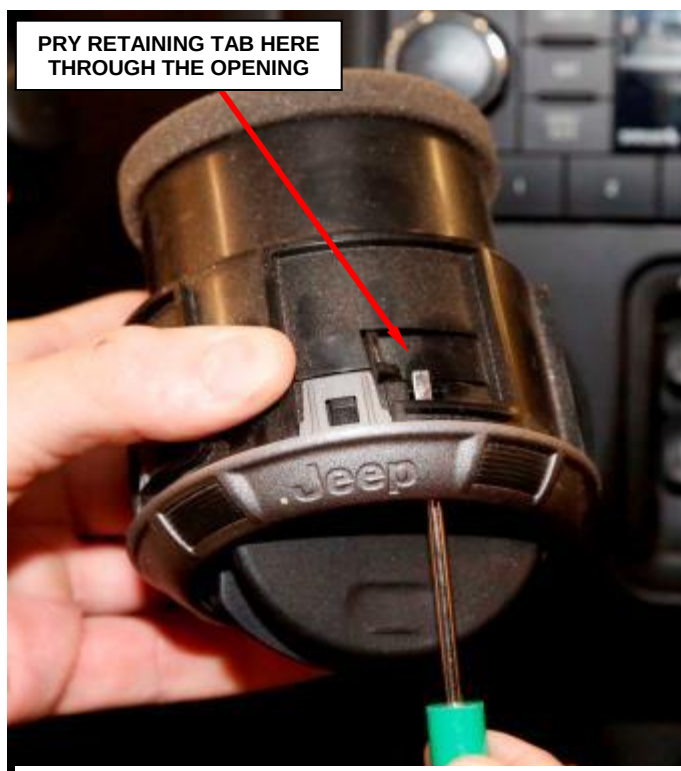
Figure 161 - HVAC Outlet Tab
