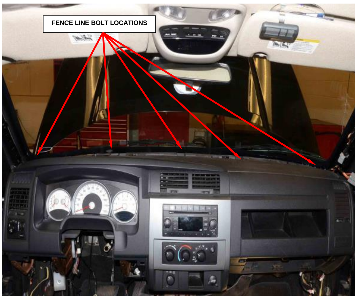
Figure 140 - Fence Line Bolts
