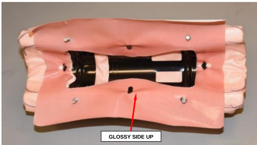
Figure 172 – Fabric Gasket to Cushion (Glossy Side Up)
