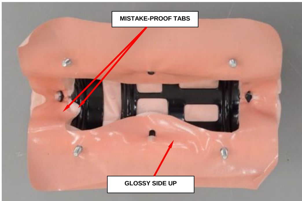
Figure 150 – Fabric Gasket to Cushion (Glossy Side Up)
