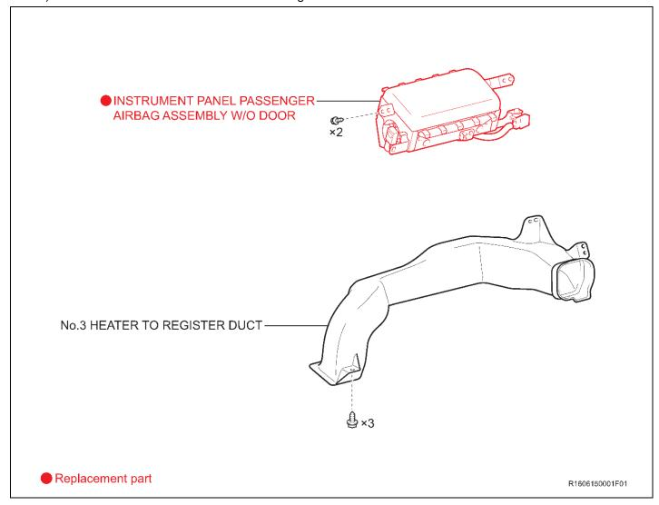
c) Remove the 4 bolts, disengage the straps, and then remove the airbag assembly.
