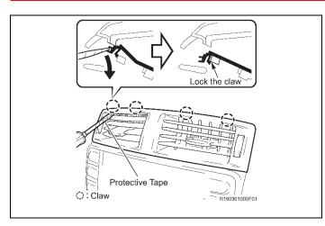
Removing the No. 3 air register
