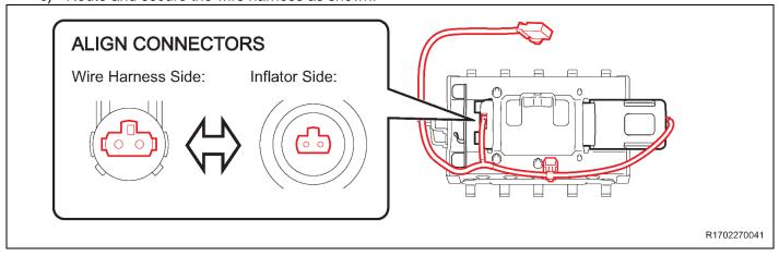
d) Fully insert the inflator and ensure that the inflator is correctly orented as shown. NOTE: DO NOT pinch the wiring between the bracket and the inflator.
