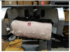
g) Mount the airbag into the mounting bracket as shown. Pass the stud on the adaptor through the hole in the middle of the bracket with the nut.
