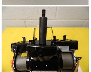
Thread the adaptor into the airbag as shown.
