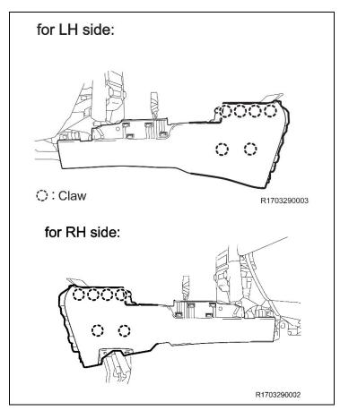
c) Reengage the 6 claws on each side of the console as shown.
