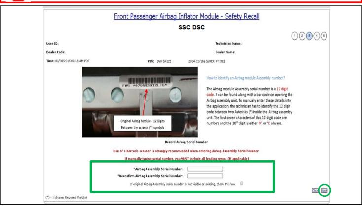
c) Check the box that states that the inflator serial number is not visible or missing.
