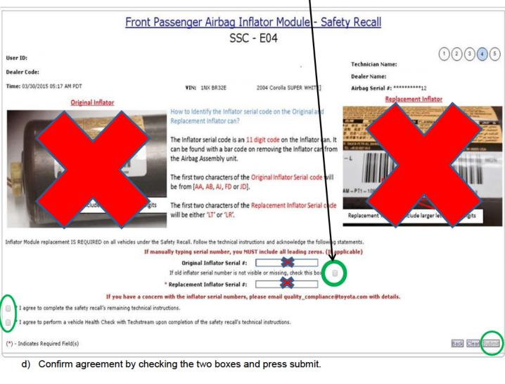
NOTE: The NEW AIRBAG ASSEMBLY serial number MUST be scanned prior to reinstallation to track the airbag to the vehicle (refer to page 14).
