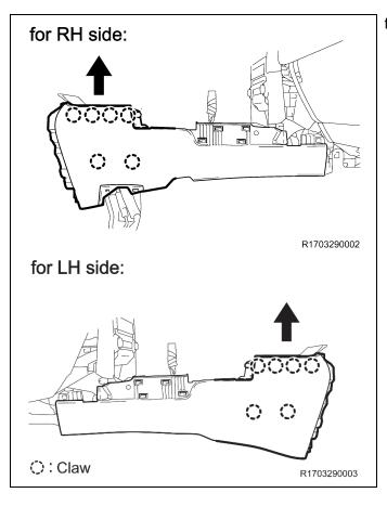
Disengage the 6 claws on each side of the console as shown.
