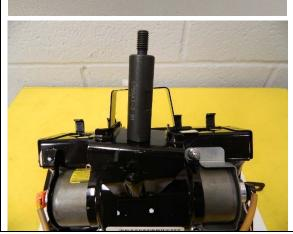
f) Thread the adaptor into the airbag as shown.
