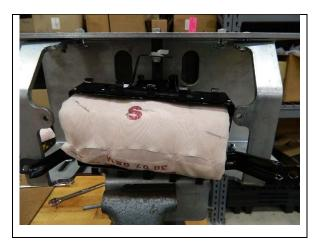
g) Mount the airbag into the mounting bracket as shown. Pass the stud on the adaptor through the hole in the middle of the bracket with the nut.
