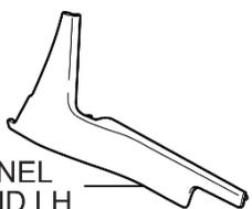
REAR CONSOLE END PANEL SUB-ASSEMBLY (Design varies depending on specifications)
