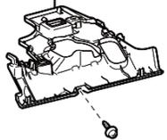
No. 2 INSTRUMENT PANEL UNDER COVER SUB-ASSEMBLY
