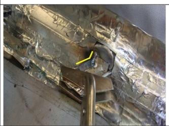
15. First, weld the left side of the bracket, progress to the top of the bracket as shown. Then continue to weld the left side of the remaining brackets as to allow time to cool.
