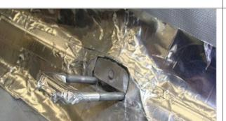
13. Prepare ISOFIX anchor for welding. Note: Area at left is example of properly prepared area. Paint on end of anchor is intact.
