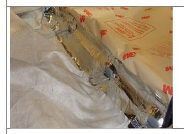
9. Install aluminized foil around ISOFIX anchors.
