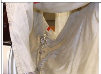
8. Protect roof liner from welding spatter.
