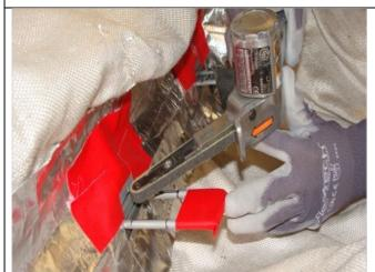
12. Remove paint from the designated areas using an abrasive belt. Only remove paint coating, DO NOT remove any metal.
