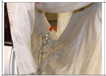
8. Protect roof liner from welding spatter.
