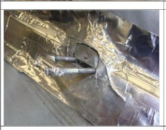
13. Prepare ISOFIX anchor for welding. Note: Area at left is example of properly prepared area. Paint on end of anchor is intact.
