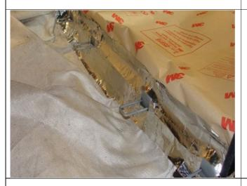
9. Install aluminized foil around ISOFIX anchors.
