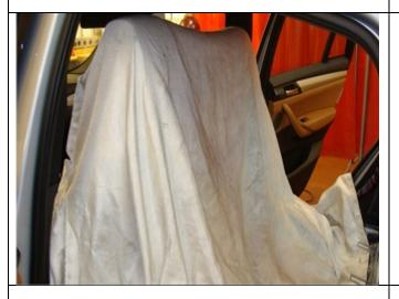
6. Cover the rear of the front seat with a welding blanket.
