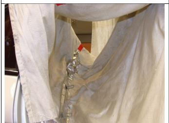
8. Protect roof liner from welding spatter.
