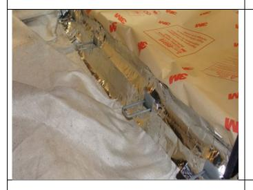
9. Install aluminized foil around ISOFIX anchors.
