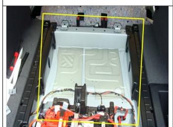
2. Remove luggage compartment floor and storage trays. Follow Repair Instruction "51 47 102 Removing and installing/replacing luggage compartment floor trim panel"
