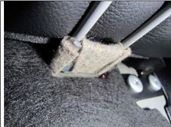
23. Lower view of felt installation.
