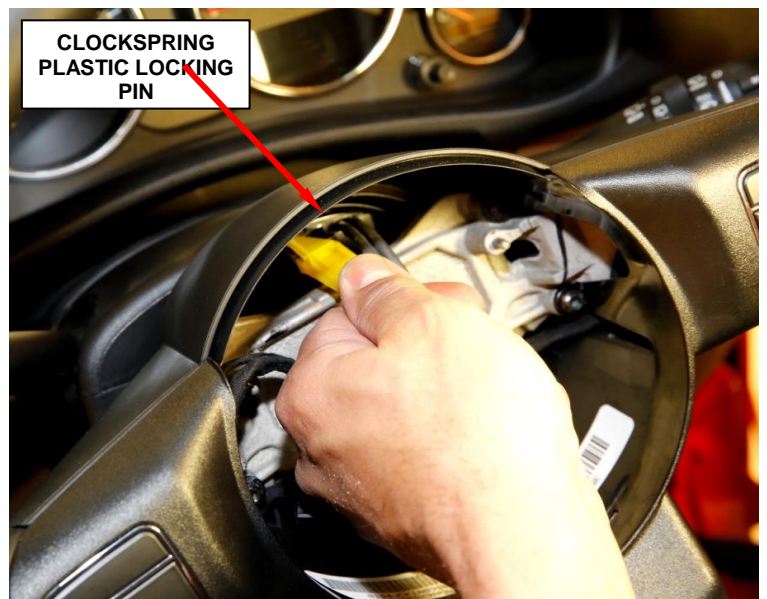
Figure 9 – Remove Clockspring Locking Pin
