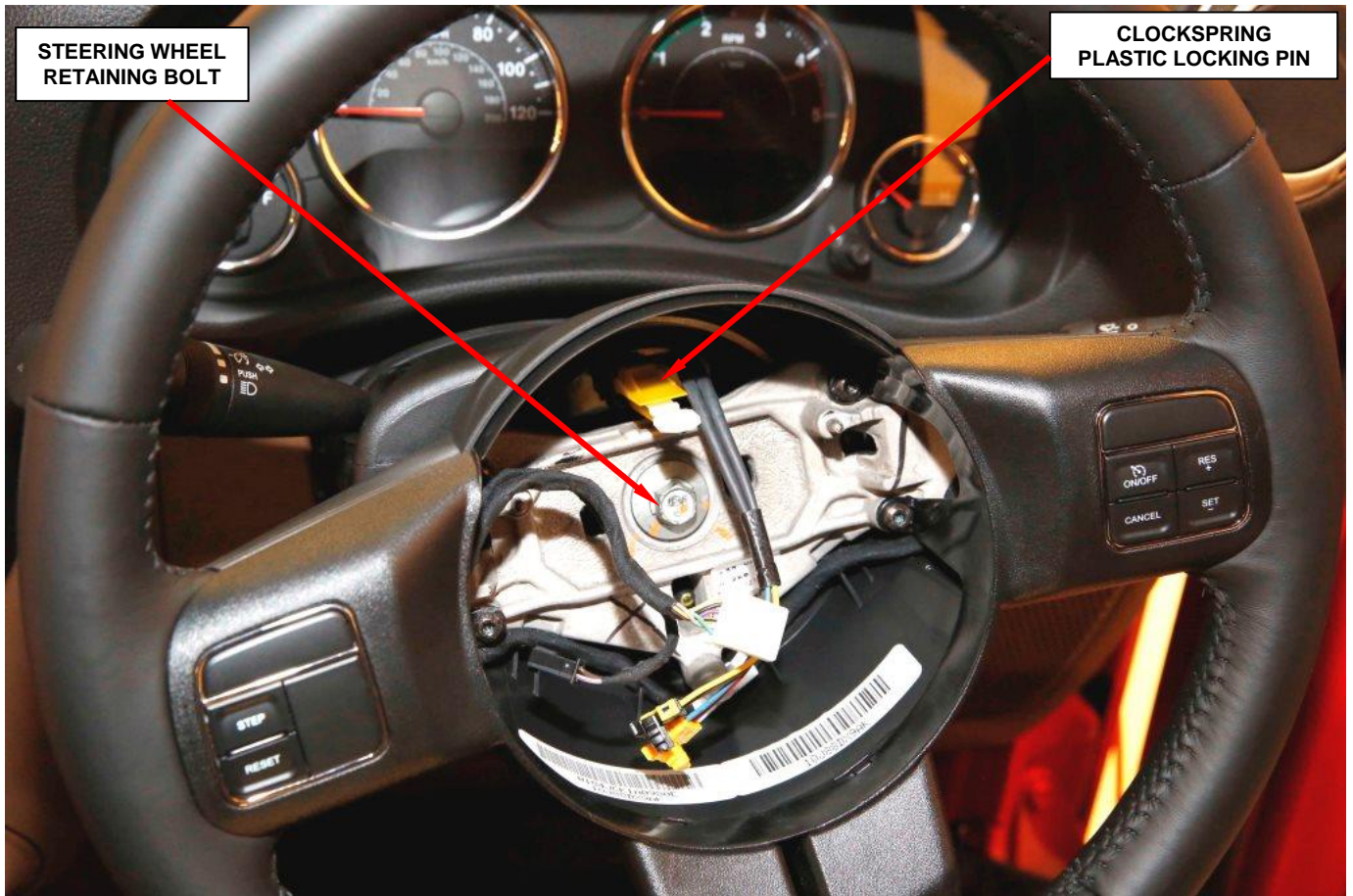
Figure 8 – Install New Steering Wheel Retaining Bolt
