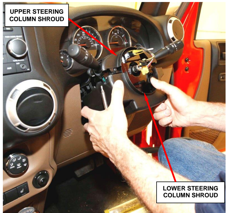
Figure 7 – Install Steering Column Shrouds
