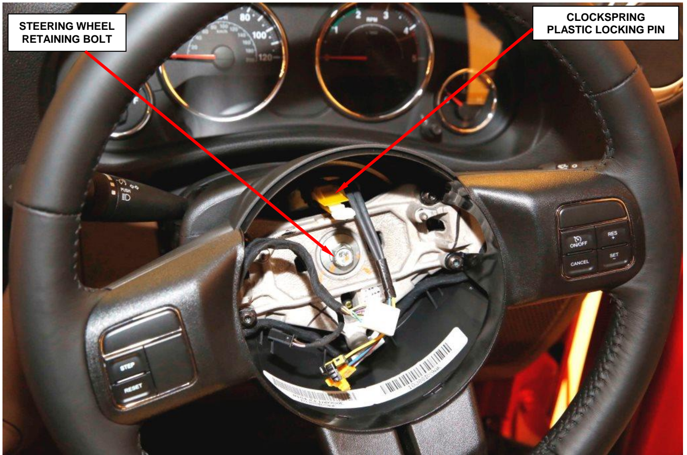
Figure 8 – Install New Steering Wheel Retaining Bolt
