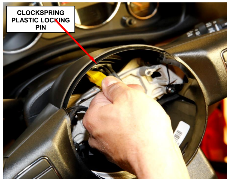
Figure 9 – Remove Clockspring Locking Pin
