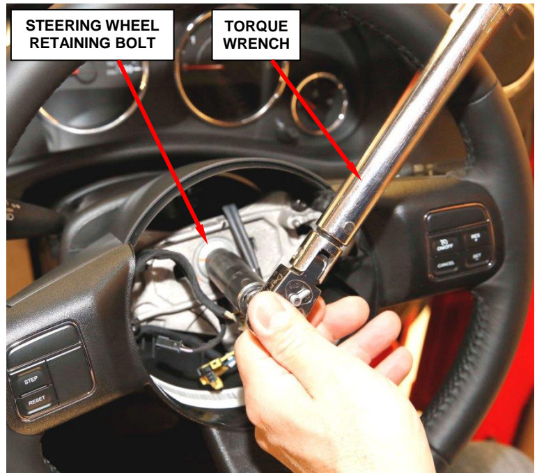
Figure 10 – Tighten Steering Wheel Retaining Bolt to 40 ft. lbs. (54 N·m)
