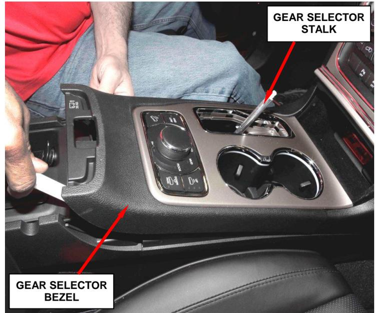
Figure 3 – Gear Selector Bezel
