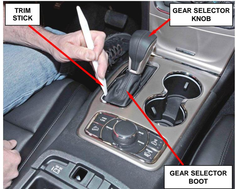
Figure 1 – Gear Selector Boot
