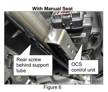
• For the manual seat, access the rear screw from behind the support tube.
