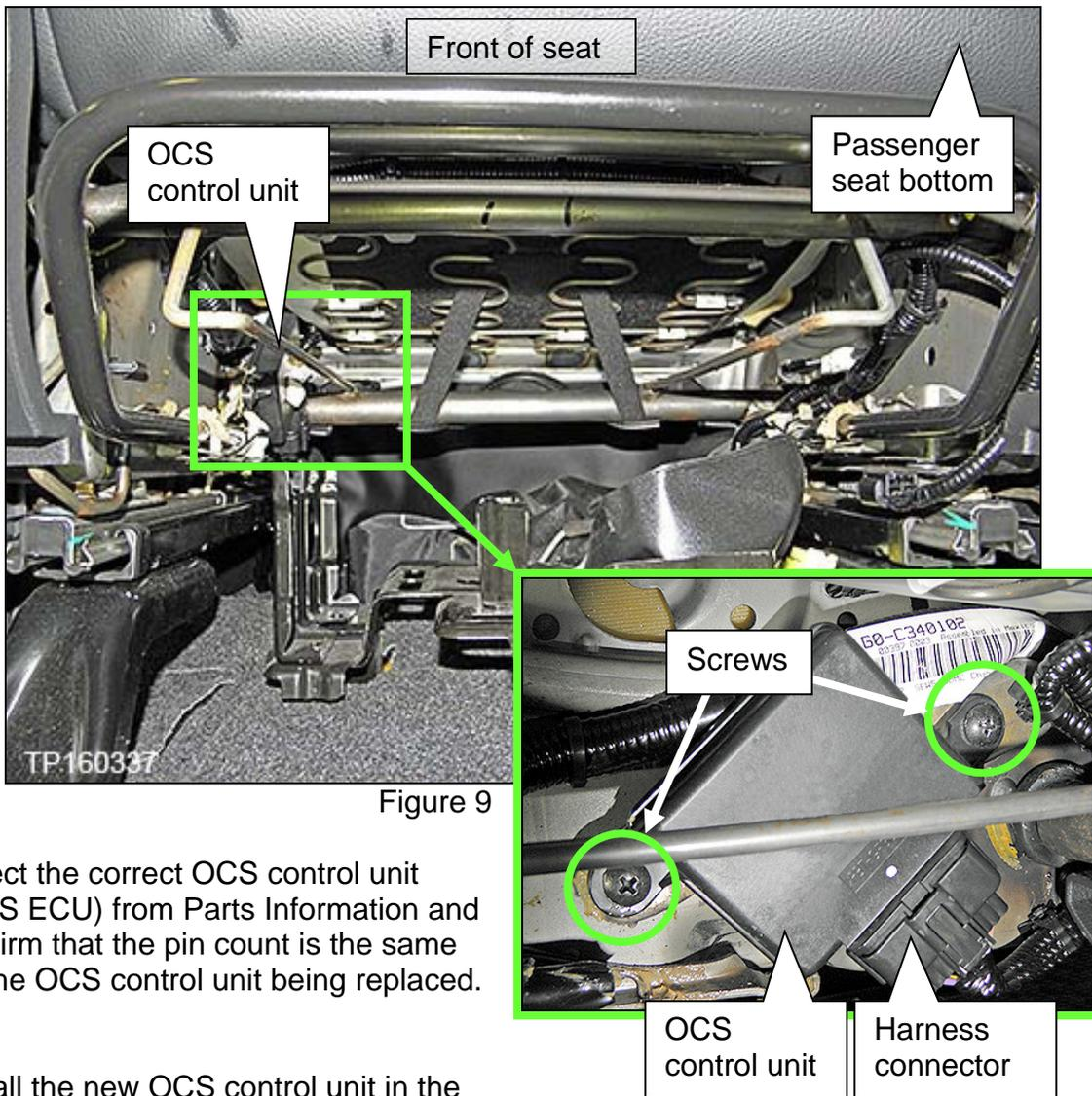
5. Select the correct OCS control unit (ODS ECU) from Parts Information and confirm that the pin count is the same as the OCS control unit being replaced.
