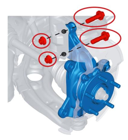
2. Clean the contact surface of both bolt and nut using a degreaser.
