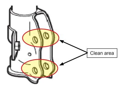
3. Install both new bolts and nuts. Use the table below to tighten the nuts to the tightening torque.
