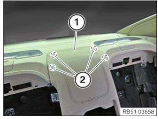
Loosen the rear console (<u>1</u>) from the clamps towards the top in this area (<u>2</u>).
