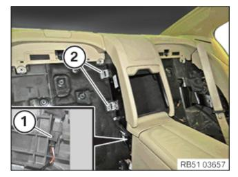
Insert the rear console (<u>1</u>) and position it on the attachment points (<u>2</u>) on the left and right.
