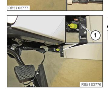
• On the left side of vehicle, tighten the screw (1).
