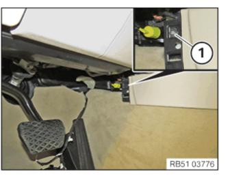
• On the left side of vehicle, loosen the screw (1).
