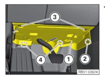
8-Removing the bottom left instrument panel trim
