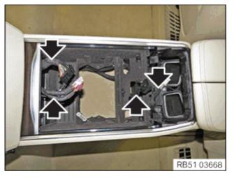
• Insert the wiring harness and secure to all cable clips.
