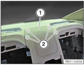
Clip in the rear console (1) into the clamps from the top in this area
