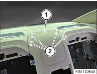
• Loosen the rear console (1) from the clamps towards the top in this area (2).
