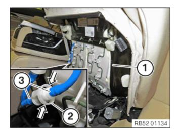
Press together the coupling (2) at the marked points and pull apart the lines (3) by gently moving them up and down.
