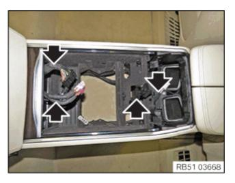
• Loosen the wiring harness on all cable clips and feed back in.
