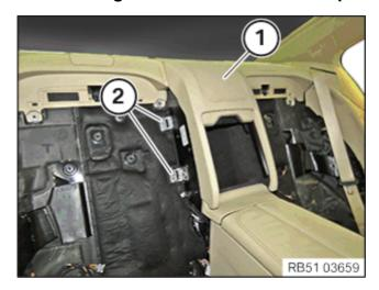
• Insert the rear console (1) and position it on the attachment points (2) on the left and right.
