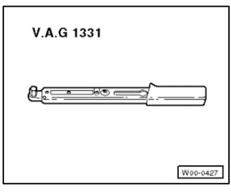
Torque Wrench 1331 5-50Nm -VAG1331 (or equivalent)
