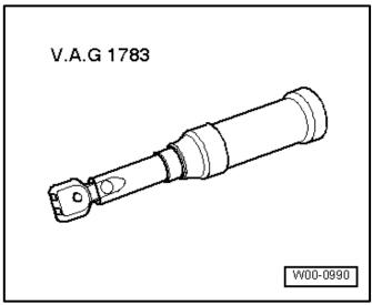
Torque Wrench 1783 - 2-10Nm -VAG1783 (or equivalent)
