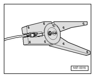
Strip the wire ends of the J583 control module harness wiring and the new connector using the Wiring Harness Repair Set - Wire Strippers -VAS1978B/3-.
