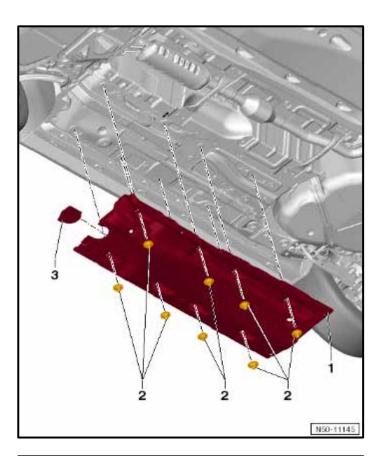
Reinstall the underbody panel <1> onto the cover <3> and reinstall the underbody cover nuts <2>. Tighten to 2 Nm.
