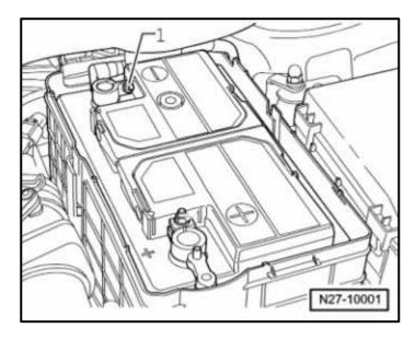
On the vehicle battery, loosen the clamp <1> and remove the battery ground cable terminal from the battery negative pole.
