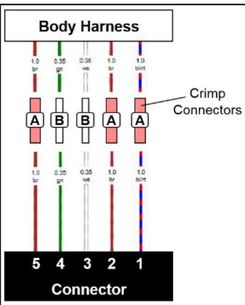
Reference the graphic to the left when connecting and crimping wiring to ensure the proper circuits are connected and the correct crimp connectors are used.
