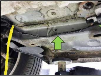
Using black insulating tape, wrap the body harness wiring <arrow>.
