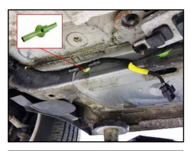
Using black insulating tape, wrap the J583 control module harness and the body harness wiring together, ensuring to reattach and secure the retaining clip <as shown>.
