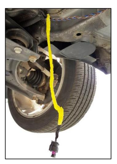
Using yellow insulating tape, carefully wrap the J583 control module harness.
