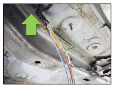
Continue to unwrap the J583 control module wiring until you reach the upper harness retainer <arrow>.
