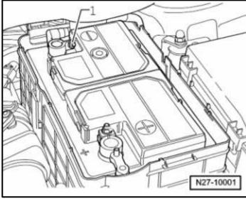
Reattach the ground cable to the battery negative terminal and tighten the clamp <1> to 6 Nm.
