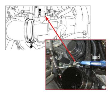
• Remove the 2 bolts securing the air intake duct to the turbocharger and remove it.
