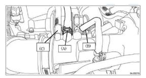
• Remove the hose clamp and the rubber intake boot from the turbocharger air intake duct. Disengage the spring clamp securing the by-pass valve to the turbocharger air intake duct as shown below.
