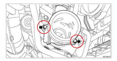
**VERY IMPORTANT:** Inspect the removed air intake duct closely for any cracking or damage. If the inspection shows the duct is cracked or has any pieces missing, the turbocharger impeller should be inspected closely for possible damage. If impeller damage is confirmed, the turbocharger assembly must also be replaced.
