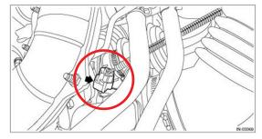
• Disconnect the PCV hose (A) and the vacuum hose (C) from the turbocharger air intake duct and remove the vacuum hose (B) from the waste gate control solenoid valve.
