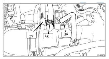
• Reconnect the wiring harness connector to the waste gate control solenoid valve.
