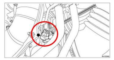
• Reinstall the undercover following the installation procedure in the applicable Service Manual.
