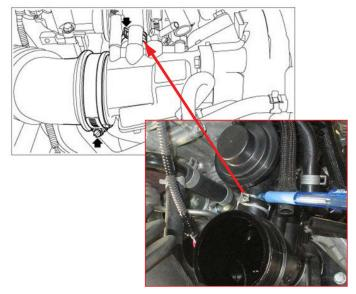
• Remove the 2 bolts securing the air intake duct to the turbocharger and remove it.
