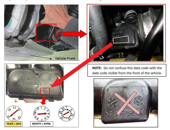
**IMPORTANT:** Only turbocharger air intake ducts with a production date of **APRIL** (Month 4), 2015 require replacement. If the production date code is confirmed to be **OTHER THAN APRIL** (Month 4), the turbocharger air intake duct does **NOT** need to be replaced.
