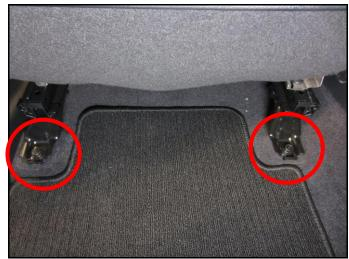
4. Use a needle nose plier to unlock the clip from the inboard side seat frame, by pinching the two locking tabs.
