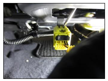
6. Use a flathead screwdriver and gently push the black secondary lock tab outward.
