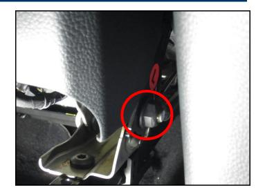
6. Remove the seat belt buckle and harness and replace with a new part.
