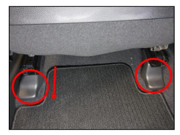
3. Remove the four driver seat bolts using a 14mm socket and ratchet.
