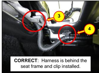
3. If the buckle harness is not installed correctly, inspect for wire damage.
