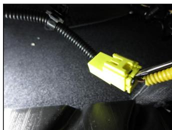
Image to the right shows the black secondary locking tab disengaged.
