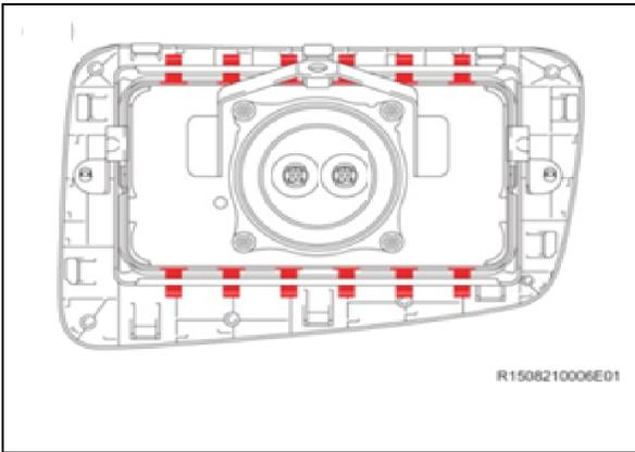
b) Reengage the tangs of the module into the door using the screwdriver with the shaft wrapped in tape.
