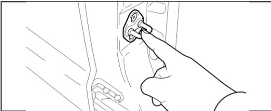
If the anti-static kit is not available, before starting work and periodically while working on the vehicle, touch a metallic part of the vehicle to discharge static electricity in the body.
