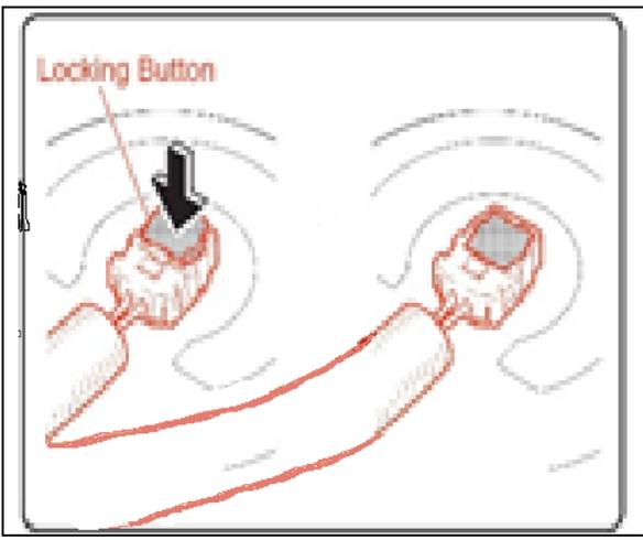
c) Connect the new harness to the new module.
