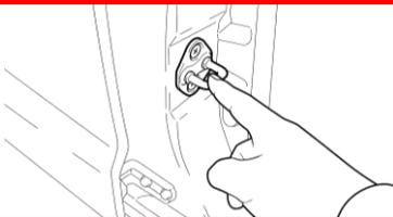
**Remember to periodically touch a metallic part of the vehicle to discharge static electricity in the body if the anti-static kit is not being used.**
