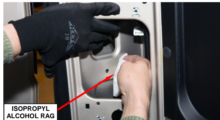
Figure 4 – Remove Residual Adhesive
