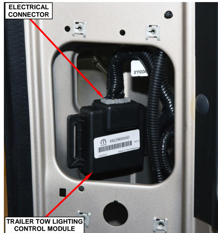
Figure 7 – Connect Electrical Connector
