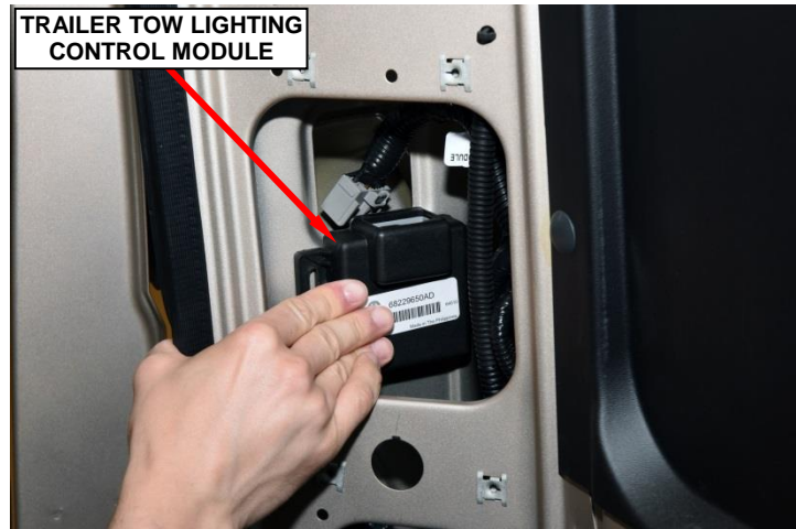
Figure 6 – Press And Hold New Module
