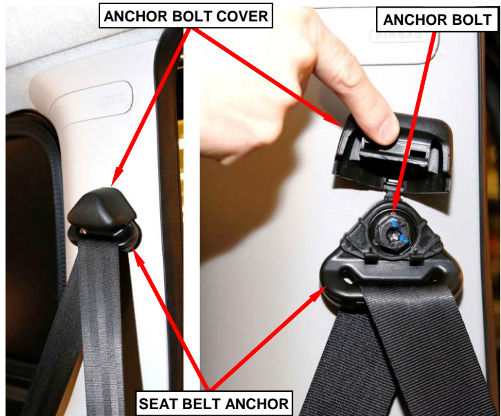
Figure 8 – C-Pillar Seat Belt Upper Anchor
