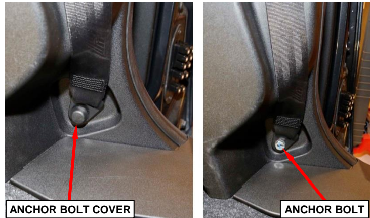
Figure 10 – C-Pillar Seat Belt Lower Anchor
