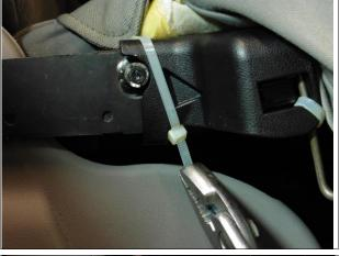
f) Using a screwdriver rotate the plastic tie locking mechanism so that it is not exposed.
