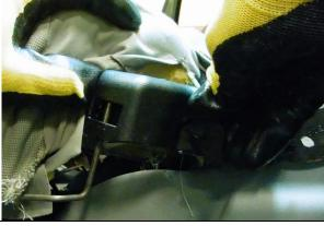
b) Engage the front tab with vertical wire of the seat frame as shown.
